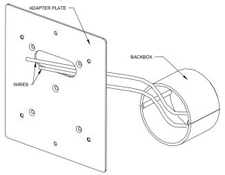
2. Secure the adapter plate to the backbox. Refer to the following diagram and table to determine which holes and screws to use.
